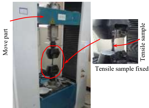
Fig. 4. Specimen in machine (tensile test).
