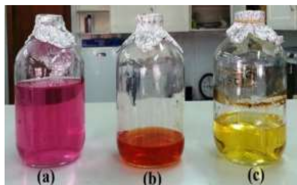
Figure 1. Different coloration of the red pigment at (a) pH 2 (b) pH 7 and c) pH 9
